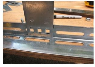
Reattach plates to angle by securing nuts and bolts. The high lift extension system is now readjusted and ready to be packaged.
