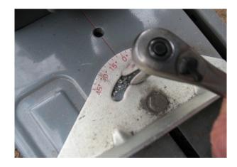
Cut tracks with circular saw. Caution: Wear safety goggles to protect against flying sparks, and be careful to keep hands a safe distance from the blade. Cut at least an inch from the end to allow for room for the angled cut; otherwise, the cut will not be even. After cutting one end, measure and cut the other, making sure they're both pitched at 4° in the same direction.
