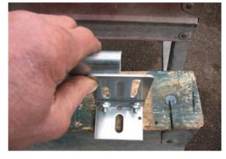
Vice grip bracket to track and drill two holes through slot onto track.
