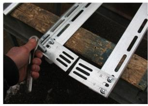
Secure center of one of the tracks to center of lower high lift plate.
