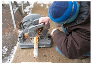
After cutting, the severed ends of the tracks will be sharp, so grind them. If you cannot get to the edge with a grinder, use a file.
