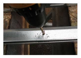
Take a precut piece of angle and file the ends. Mount lower numbered high lift plates to the bottom of the angle and secure with 5/16" carriage bolts and flange nuts.
